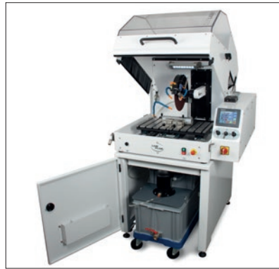
Support cabinet with integrated cooling system 60 litres.
