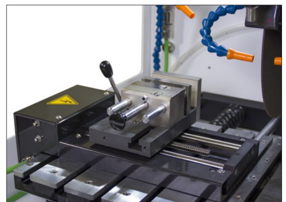
X axis table automatic or manual, stroke 150 mm.
